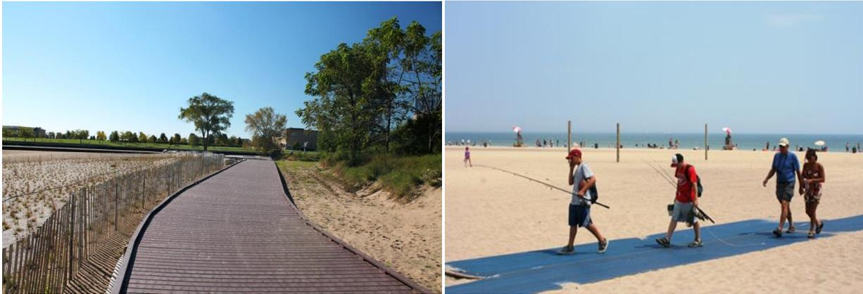
**Figure 11:** Left: Defined pathways protect vegetated areas during the establishment phase (Simmons Island Beach, Kenosha, WI), Right: Example of Mobi-Mat™ pathway (North Beach, Racine, WI).
