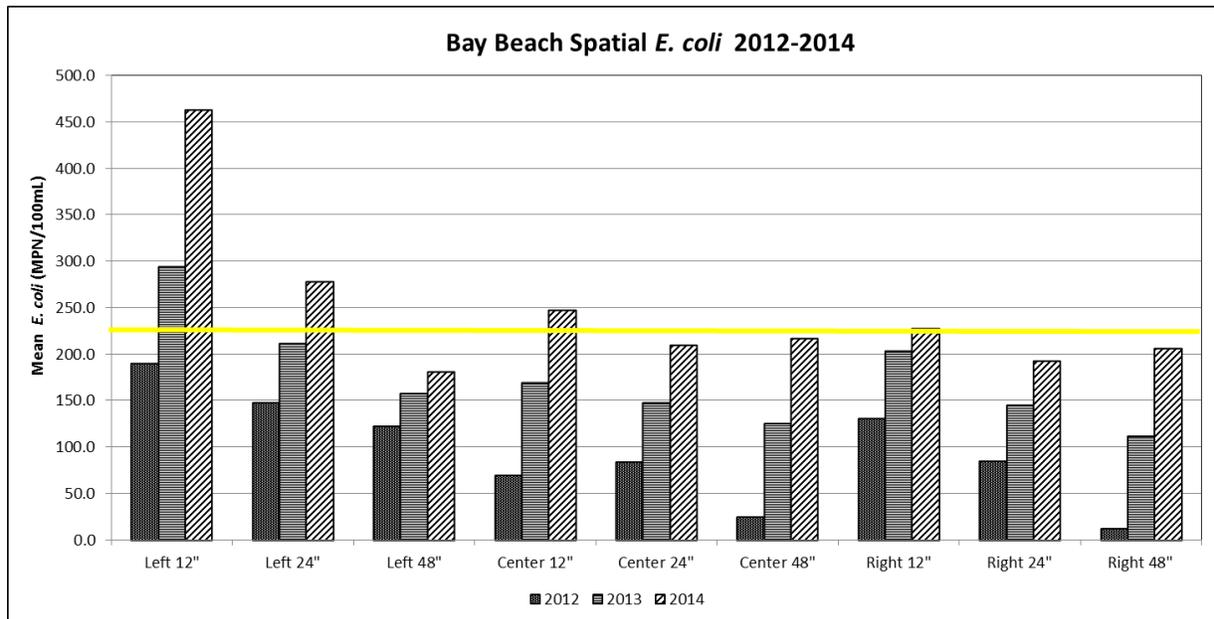
**Figure 2.** Routine Sanitary Survey average log *E. coli* results for Bay Beach over three years of sampling all located on Lake Michigan (2012 n=63; 2013 n=234; 2014 n=207  $p < 0.05$ ). The yellow line indicates the *E. coli* exceedance level for a beach advisory at 235 MPN/100 mL. If *E. coli* exceeds 999 MPN/100mL the beach would be under a closure (line not shown).
